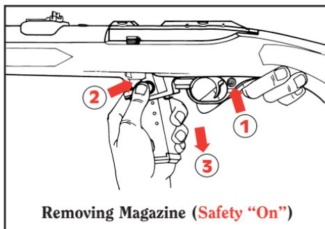
Figure 3. **The safety should be “on” when the magazine is being removed or inserted.** When the magazine latch button is pushed in, the magazine is released. Depress the latch with the thumb and at the same time grasp the magazine between your fingers and draw it downward out of the gun. **REMEMBER to check to be sure the chamber is empty after removing the magazine!**
