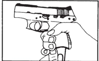
2. Pull SLIDE fully to the rear and push up the SLIDE CATCH LEVER.
