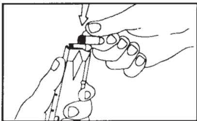
3. Hold the pistol with one hand keeping your finger away from the **TRIGGER**. With the other hand pull the **SLIDE** to its limit and release it. You may depress the **SLIDE CATCH**, and the **SLIDE** will go forward under **RECOIL SPRING** pressure and will insert one cartridge in the chamber.
