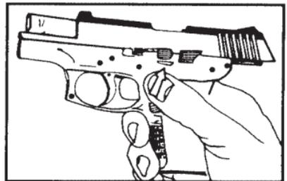
3. With left thumb, rotate SLIDE DISASSEMBLY LATCH clockwise until it stops.
