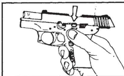
5. If you want to stop shooting before firing the last cartridge of a magazine, push the safety lever in the up (on) position.
