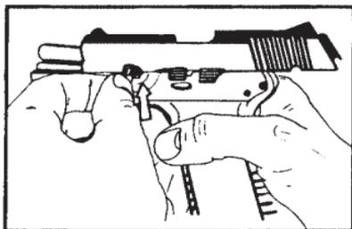
5. Carefully release SLIDE CATCH, and with SLIDE under full control, pull SLIDE forward off of frame.
