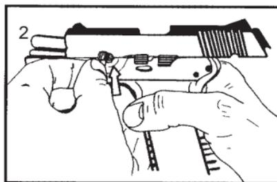
Insert the take-down pin once the slide is in position to line up the barrel with the hole, and gently push in. A click will indicate the pin is secured in place.
