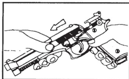
4. Slightly press the RECOIL SPRING GUIDE. Lift and remove it carefully.
