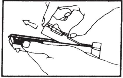
5. Press LOCKING BLOCK PLUNGER (PT-92 C-D, PT-92AF-D, PT-99 AF-D, PT-100 AF-D AND PT-101 AF-D)
