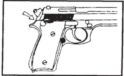
On **PT938** pistols it is necessary to press slightly down on the barrel while assembling the slide on the frame.
