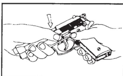
3. Pull forward the SLIDE-BARREL assembly.
