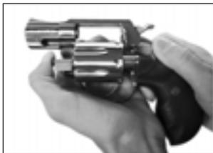
To unload, open the cylinder as previously described under “loading”. Elevate the barrel, with the cylinder fully open, push rearward, smartly on the front of the extractor rod, this will extract all cartridges so that they will either drop out
